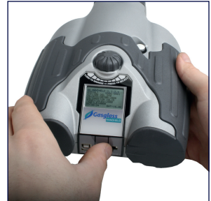
4. Power the device on using the ON/Off switch
